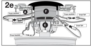
Slide the remote receiver (**F**) onto top of the canopy mount (**A**). Connect wiring harness from receiver (**F**) to wiring harness from fan body (**C**). Connect wiring harness from canopy mount (**A**) to wiring harness from receiver (**F**).
