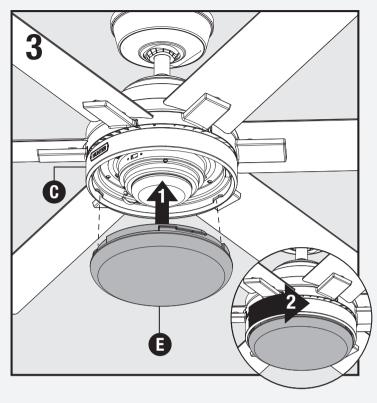
Align, lift and twist to lock light cover (E) to bottom of fan assembly (C).
