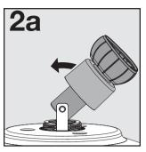
Rotate the downrod into an upright position.
