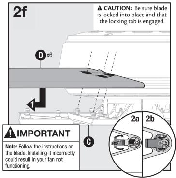
Insert the blade iron posts (**C**) completely through the larger end of the blade key holes (**D**). Slide the blade (**D**) away from the blade posts (**C**) to engage the keyholes. Lift over and lower the locking tab. Press and insert to engage the locking tab. Repeat for remaining blades (**D**).
