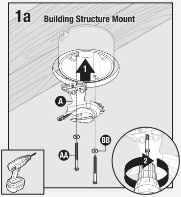
Using wood screws (**AA**) and washers (**BB**) included, install canopy mount (**A**) through box outlet into building structure. Drilling 9/64" pilot holes in building structure will aid in securing canopy mount (**A**).
