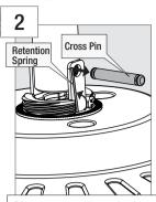
Disengage retention spring by pulling away from rod. Then remove cross pin from downrod. Remove downrod assembly from pivot assembly.
