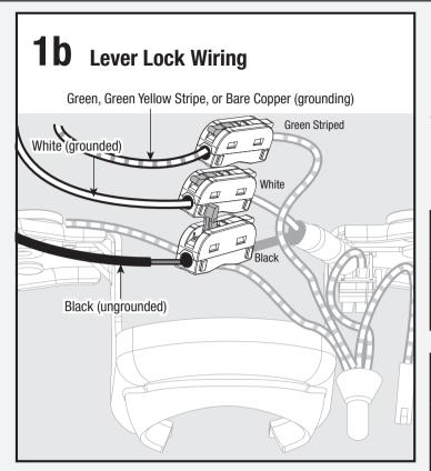
Connect wiring from ceiling to lever lock wiring (on side of canopy mount) by lifting lever and inserting wire. Lift lever on connector until fully upright to open. Insert stripped wire and secure by lowering lever. Make sure no bare or uninsulated wire is exposed.
