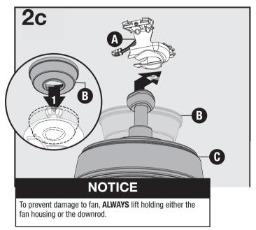
Install snap-on canopy (**B**) over downrod on fan body (**C**). Place the down rod ball into the slot in canopy mount (**A**) with built-in ceiling bracket.
