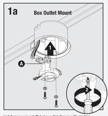
Install canopy mount ( $\bf A$ ) to box outlet. Secure with machine screws and washers (provided with outlet box).
