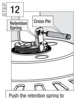
Push the retention spring to the side to allow cross pin access. Place cross pin through downrod assembly and the pivot bracket. Place retention spring into the groove of the cross pin.
