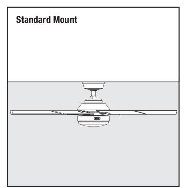
This installation is for  ${f flat\ ceilings}$  using the short pre-installed downrod ceiling fans.
