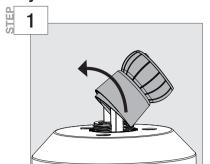
In order to change the length of downrod, the pivot assembly needs to be disengaged. Rotate the downrod into an upright position.
